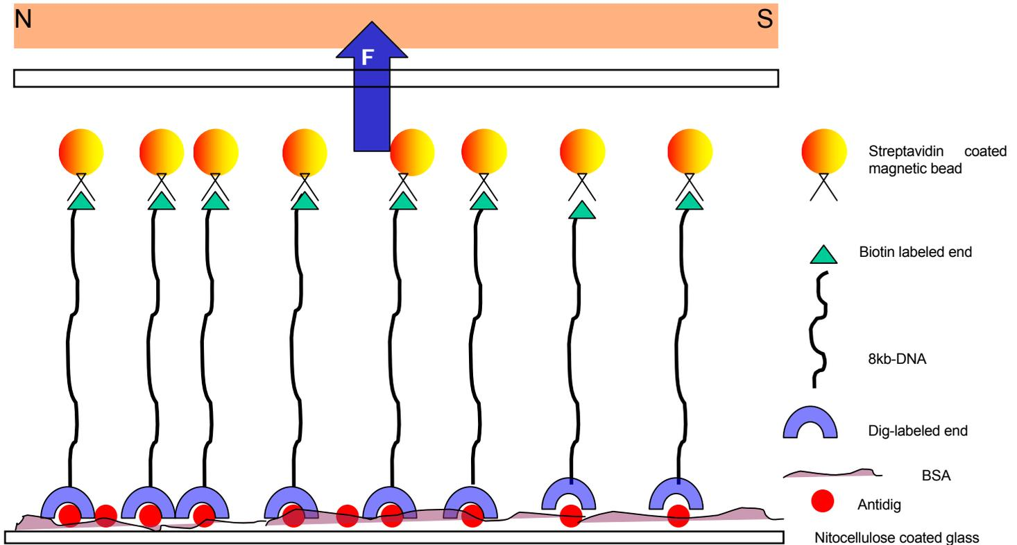
**Fig. 1:** Schematic representation of the set-up used
