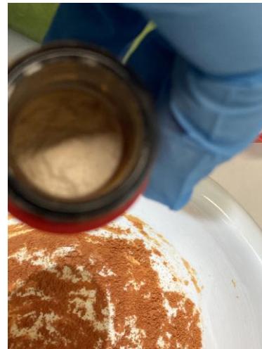
Fig. 6: Polymeric l-dopa compound which has a beautiful orange color. L-dopa is a white solid as can be seen in the inside the bottle (above)
